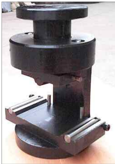
Compression shear adhesion strength jib for adhesives (ISO13007-2)
