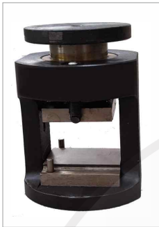
3-point flexure fixture for grouts (ISO13007-4)
